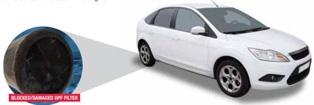
**Diesel Particulate Filters (DPF)** work by filtering soot particles from the exhaust to minimize soot emissions into the air we breathe. However, the DPF needs to be regenerated in order to stop it from eventually blocking.
